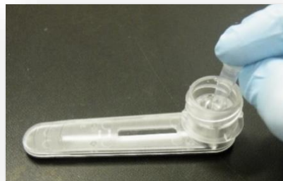
2. Put PCR tube into Cassette
